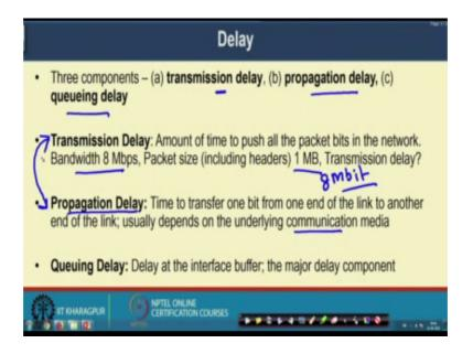
Now, coming to delay in network there are three different types of delay or you say that; there are three components of delay, the first one is the Transmission delay then we have the Propagation delay and the third one is the Queuing delay.
