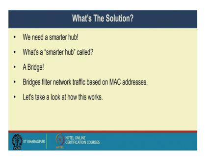
So, the solution is whether we can have a smarter hub or bridge. So, bridge filter traffic based on the MAC address; that means, as every NIC have a unique MAC address or every system has a unique MAC address. So, they filter traffic based on the MAC address. So, how it looks like?
