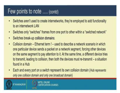
Switches are not used to create internetworking so, that is for router. They are employed to add functionality to the internet LAN. So, switches breaks up collision domain. It switches frame from one part to the other part in a switch network so to say that is why the switch.
