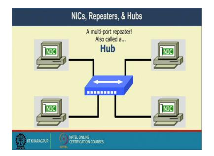
And if I want to connect more than two things, then I require a multiple repeater or popularly we called as a hub these are all layer one devices. So, it is only amplifying the signals and type of things right.
