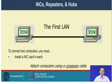
So, if I have two computers with NIC cards, the first LAN how to connect is connect to in kind of either cable; only thing that should be a crossover cable; that means, the transmitter or TX of one should go to the RX and RX of the others should go to that TX. So, it is a crossover cable or what sometimes what we say cross cables right.
