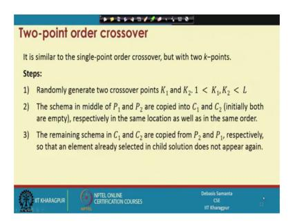
So, it is just procedure of 2, I mean deciding instead of 1 K values we have to decide 2 K values and these 2 K values are denoted K1 and K 2; the 2 values are the same as it is in case of the previous 1 scheme; that means, the values of the K values should be in between 1 and L.
