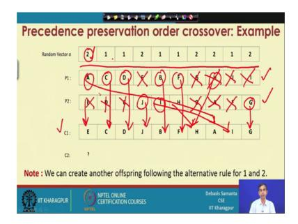
So, this is the vector V, with size same as the parent P1 and parent P2 and will see how the C1 can be obtained. So, here the idea is that if P is 2, I mean if the current value is 2 then we will copy from P2 and if the current value 1 will copy from P1, so it is like this. If 2 it is there, so this is copied; here is 1 is there so will copy from this one. Now, when will copy E so, all E should be deleted both from P1 and P2, so it is been copied there.
