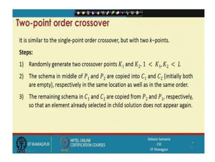
So, we assume these are the 2 solution appearance P1 and P2 and then a random K point is decided, this is the K point from where the left schema and right schema. So, this party is the left schema and this is the right schema for the parent P1, similarly this is a left schema for the parent P2 and the right schema for the parent P2.
