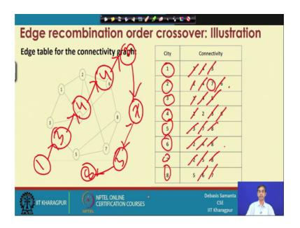
Then, the next city we have to select from city 1 we can go 2, 4, 3. Now, in case of 2 the connectivity is 3, in case of 4 it is again 3 connectivity that there in case of 3 it is 4, so we should select the minimum connectivity that mean 3 in this case, so we will select the next city as 3 and then as 3 is connected. So, we will remove this 3 from every occurrences in the connectivity matrix that mean 3 has been covered.
