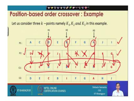
So, let us explain illustrate this technique with an example, will consider this is the P1 and another chromosome P2 and here we consider 3 points K points, these are called the K1, K2 and K3. So, account the scheme the first scheme will produce a C1, so this D 1 is copied here and then this B1 is copied here and then this H1 is copied here.
