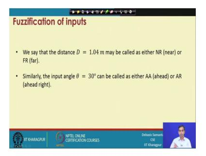
So, we can understand that the D distance 1.04 can be called either NR or FR; that means, they belongs to the two fuzzy state with different membership values similarly the angular orientation theta 30 degree can be called as either ahead or ahead right with
