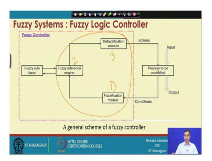
Now, so first will discuss the fuzzification module because the input it will take the data that is required to control the system and the fuzzification module will produce an output which will be used by the fuzzy inference engine. So, we should learn fuzzification module first then we will be able to discuss about the fuzzy inference engine.
