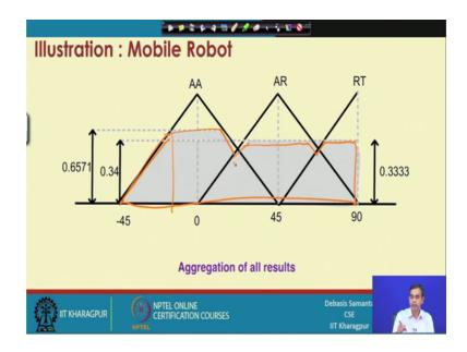
Now, I can give an example here for example, if we plot the 4 different output into the same graph the graph will look like this. So, it is basically this is the graph than this graph then this, then this, then this, then this. So, this is the output graph actually for the 4 rules related to the input x and theta, x is 1.04 theta is 30 degree.
