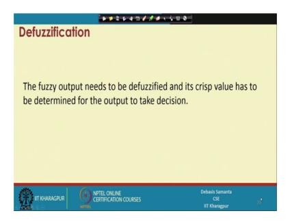
So, fuzzy outputs needs to be defuzzified and the creeps value has to be determined for the output to be taken. In this current context in the current context, this is the input here this is the input and this is another input and then output is basically delta regarding that in which direction it should move.
