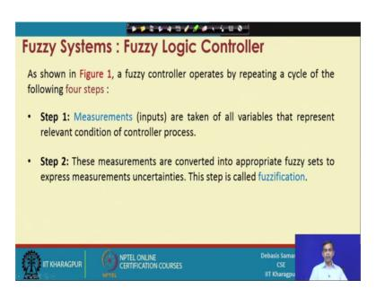
Now, I will just little bit a brief detail about the different processes involved. So, for the fuzzy logic controller is concerned it is basically a cyclic process it will take an input it will decide what exactly the control to be decided producing output take another input and output, is a cyclic method.
