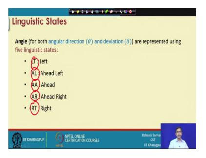
Now, similarly the angle that is the direction of the robots with respect direction of an object with respect to the robot or the deviation of the robot can be describes again in terms of 5 different linguistic states. That we have discussed about here the 5 linguistic states are left, ahead left AL, ahead and ahead right AR and then right.
