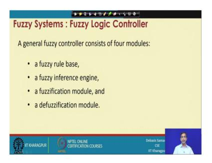
So, for the fuzzy logic controller or a fuzzy system reason is concerned we have to just design these 4 components then system will be built up.
