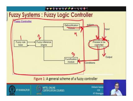
Anyway, for the fuzzy logic controller is concerned this diagram basically saw the overview of a fuzzy controller system and if we see it carefully. So, the fuzzy controller this is the portion of the fuzzy controller right and this is basically an external interface with the outer world. So, these are the basically fuzzy world and this is basically the crips world we will come into this portion later on.
