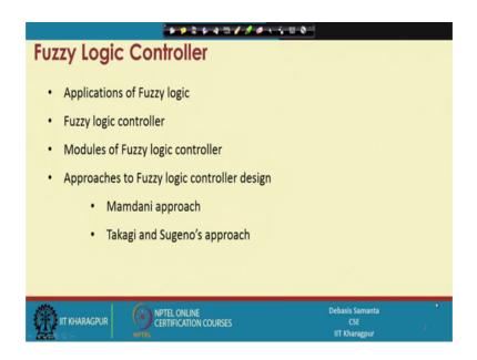
So, actually we are going to discuss about how a fuzzy logic controller can be can be designed and so for the fuzzy logic controller design is concerned they are broadly two approaches are known the first approach is called Mamdani approach and the second approach is called Takagi Sugeno approach.
