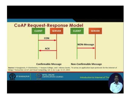
So, basically when we look at CoAP confirmable message, this is how it works. So, CoAP is basically a connection between the client and the server in a resource constraint
