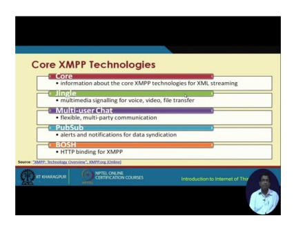
So, XMPP basically helps in doing this. There are few core XMPP technologies, one is the core technology which provides information about the core XMPP technologies for XML streaming, then we have jingle which is used for multimedia signaling with the help of voice you know wherever there is multimedia resources, such as voice, video, file transfer etcetera, it can help in signaling jingle multi-user chat.
