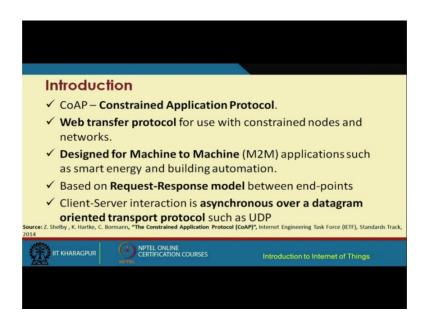
This protocol is particularly used for web transfer and by web transfer I mean very similar to the http, but web transfer in the context of constrained networks resource, constrained networks with nodes which are constrained with respect to different resources, such as limited energy or power supply, limited computational resources, limited communication resource, limited bandwidth environment and so on.
