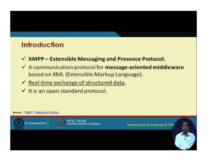
The full form of XMPP is Extensible Messaging and Presence Protocol. So, it is a message oriented middleware that is based on XML, whereas XML is particularly used for unstructured data. XMPP is useful for real time exchange of structured data and it is an open standard protocol.
