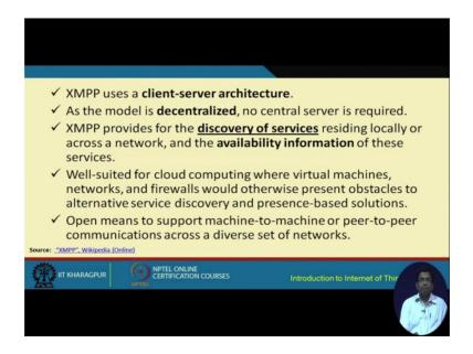
So, XMPP uses a client server architecture, it uses a decentralized model meaing that there is no server that is involved in the message transfer and it provides facilities for discovery of messages which are residing locally or globally across the network and the availability information of these services.
