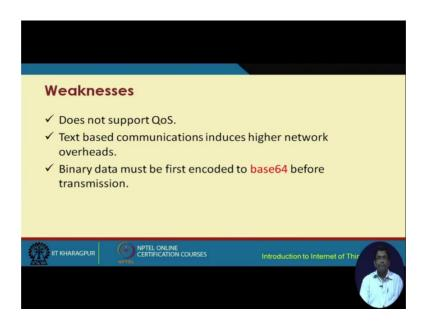
There are different weaknesses as well of XMPP protocol. It does not support QOS, text based communication including you know Higher Network Overheads are involved in the use of XMPP. So, it is not good for text based communication.
