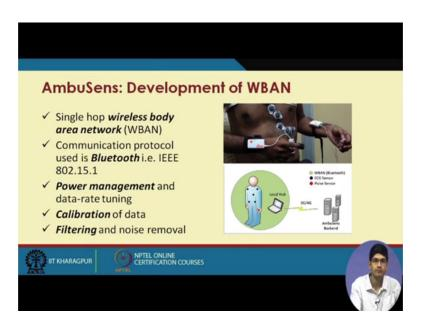
The sensing layer of the AmbuSens project consists of different wireless sensors which sample the physiological data coming from the patient and using internet of things communication technologies such as Bluetooth, Zigbee among others the data is sent to a local herb or a local data processing unit where the data is aggregated and sent further for processing.
