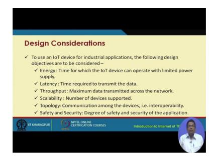
There are different design considerations for building IIoT, to use an IoT device for industrial applications these design objectives have to be considered. Energy is paramount energy with respect to the time for which the IoT device can operate with limited power supply. So, we have limited power supply and we want to extend the lifetime of the IoT device that is installed that is fitted with an industrial machine.
