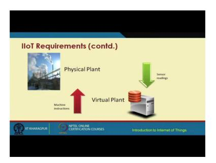
So, what we what is required is to have a virtualized version of a physical plant. So, through IIoT systems what we are trying to build is a virtualized plant corresponding to a physical industrial plant. So, these physical plant and the different machines in the plant are fitted with different sensors which throw in lot of data the sensors readings, and from
