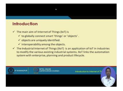
So, let us try to understand IIoT vis a vis IoT, as we have already understood through the previous lectures that the main aim of IoT is to interconnect different things and these things are different objects on the smart objects. So, what is required is to globally connect these smart object or the things so that the objects are uniquely identified and they are able to interoperate between themselves.
