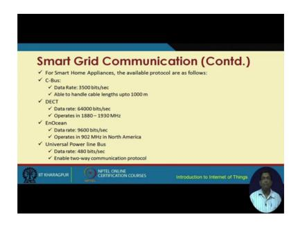
So, for smart grid appliances the available protocol that are used are C-Bus DECT, the EnOcean and the universal power line bus and I am not going to go through, but the corresponding data rate.
