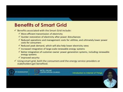
There are different benefits of smart grid; one is that it is possible to more efficiently transmit electricity than the traditional one traditional electric grid, it is it has quicker
