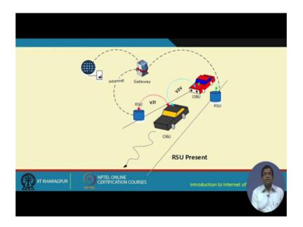
So, these are the 2 scenarios that are depicted over here that I just mentioned here is a scenario of the RSU being present and when the RSU is present you know. So, RSU has the internet connectivity via the gateway and that internet connectivity basically helps to have V2I and V2V communication.
