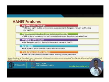
So, high through put is achievable in mobile environments using VANETs. And also low latency can be guaranteed in mobile environments in VANETs. VANET basically has different features. It has a highly dynamic topology, where the vehicle vehicles are highly mobile and they are changing their position. And the network topologies come continuously the brake and they make continuously. So, you have a highly dynamic breaking making kind of topology which is done continuously.
