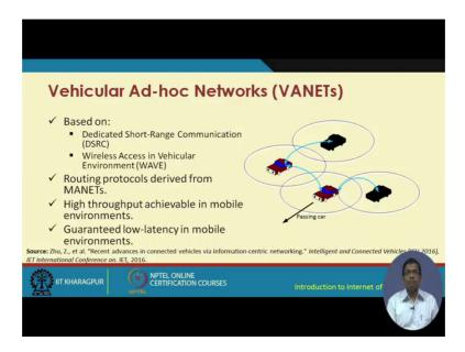
So, we are talking about vehicular ad hoc networks which is based on dedicated short range communication DSRC. And the wave protocol which is wireless access in vehicular environments the wave protocol.
