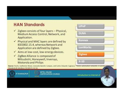
So, I am not going to talk about in too much detail here. But from a home area network perspective ZigBee is very commonly used. It has the different layers the physical layer, the mac layer, the network, layer and the application layer as you already know. By virtue of your existing knowledge of ZigBee in the module one of this course.
