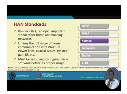
Then we have this Konnex standard in short it is also known as the KNX standard, which is an important standard for home and building networks. Which utilizes the full range of home communication infrastructure including power lines, coaxial cables, twisted pair, RF etcetera. When whatever is existing those existing infrastructure the communication infrastructure at utilized in Konnex. And this must be set up and configured via a software before it is proper usage.
