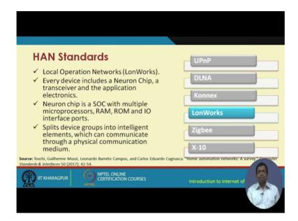
Then we have the LonWorks, local operation networks LonWorks, where every device includes a neuron chip. You know, LonWorks has different devices which include something known as the neuron chip which has a transceiver and the application electronics.
