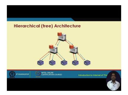
So, this is the flat architecture then we can have different other architectures this is the hierarchical or the tree architecture and these I do not need to elaborate further, but it is quite obvious we have these different switches and hierarchically they are placed within the controllers are placed and connected to these different switches in a tree like fashion.
