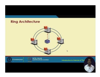
And we have this packet in message and the corresponding flow rule coming back for each of these connectivities then have the ring architecture. In the ring architecture we have a similar kind of thing, but we have to keep in mind that in the ring architecture. So, basically these controllers are placed in a ring like fashion we have multiple controllers like this placed in ring like fashion, but a particular switch is connected to only one controller in this version.
