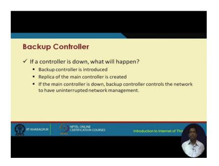
So, in such a case it is a centralized control and dividing into different sub networks are having a controller corresponding to it will be distributed solution there is also a concept of backup controller. So, if the primary controller is down then the backup controller takes over.
