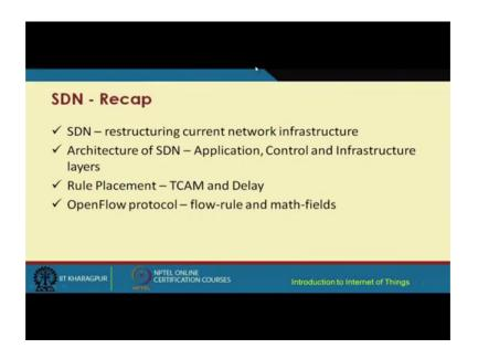
So, we have just as a recap we have already in the first part of SDN. We have understood the basic concept behind SDN the architecture of SDN the rule placement problem and the tradeoff between TCAM limitations limited memory TCAM memory and the delay. And we have also understood the open flow protocol and flow rule.
