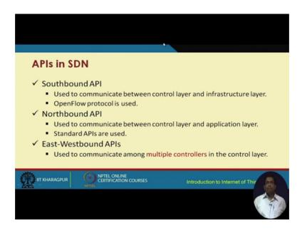
And the math rule math fields in the open flow protocol. So, in SDN between the data plane and between the data plane and the control plane we have an API and another API between the control plane and the application plane.
