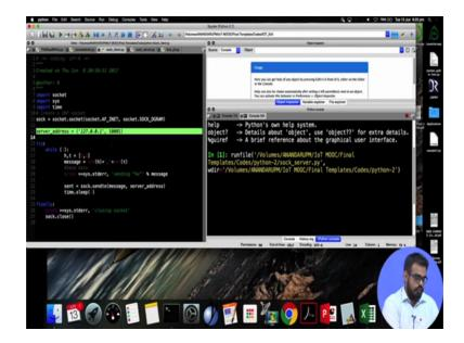
So, till this part the socket operations take place and within this the data read write operation take place, similarly for start I will get the server running. So, it does not show anything because it is expecting data from a client. On the client side, I give the same loopback address as the server, then the same port number. It is very important to have the same port numbers.
