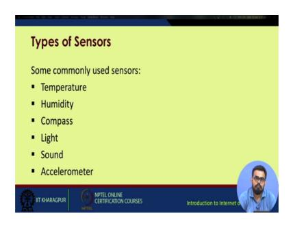
So, there are few common type of sensors we actually use with IoT they include temperature sensors, humidity sensors, compass or direction sensors light sensors, sound sensors accelerometers or mission sensors.
