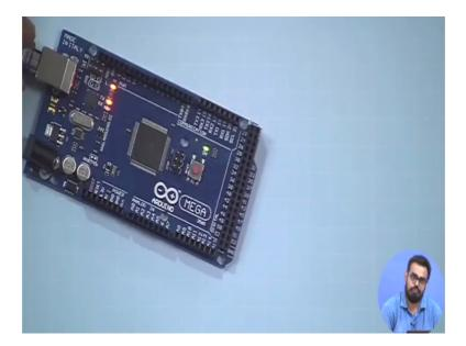
Now, we are using and Arduino at mega; so, Arduino mega. So, in the market you can just get it by the name of Arduino mega or mega 2560. So, its bit bigger than your traditional Arduino
