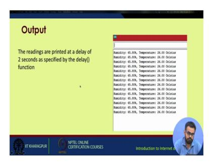
So, this is the output we are expecting like humidity is giving in percentage and temperature in degree Celsius, and these each row is separated by time duration of two seconds. So, after every two seconds your temperature readings and humidity readings are getting updated.
