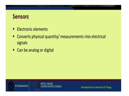
So, first of all as we have already learned by now; sensors are basic electronic elements they convert physical quantities or measurements into electrical signals and more or less sensors can be classified into either analog or digital sensors.
