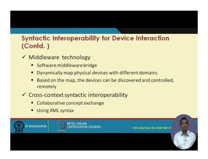
Middleware technology, so this middleware technology is sort of like a software middleware bridge, which dynamically maps the physical devices with the different domains and based on the map the devices can be discovered and controlled remotely. Then we have the cross context syntactic interoperability, which concerns collaborative concept exchange and using xml syntax.
