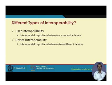
So, what is required is to have different types of interoperability, and these interpretability issues of different types have to be handled in different ways. User interoperability is between a user and a device. Device interoperability is between two different devices.
