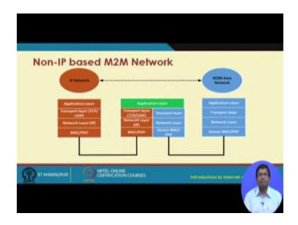
So, this is a scenario of non-IP based M2M network. So, here what we see is as you can see over here we have a non-IP based M2M area network and here we see an IP based network. And this application layer basically seamlessly integrates these two application layer basically seamlessly integrates the IP network and the M2M network in this manner.
