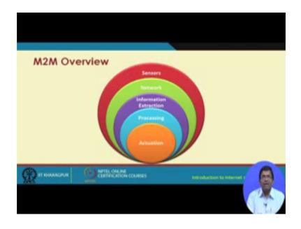
So, in M2M when we are talking about M2M, we are talking about sensors, sensors producing data through the network, information is extracted out of the data that is received, it is processed and if required some actuation is done maybe opening of the valve in an agricultural field if the soil moisture level has gone down.
