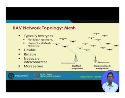
In a mesh topology, a mesh kind of topology is formed. And one of these nodes in this mesh is going to connect to the ground station like this. So, we have this unit of the mesh and this is repeated and this kind of architecture this kind of topology is; obviously, quite scalable.
