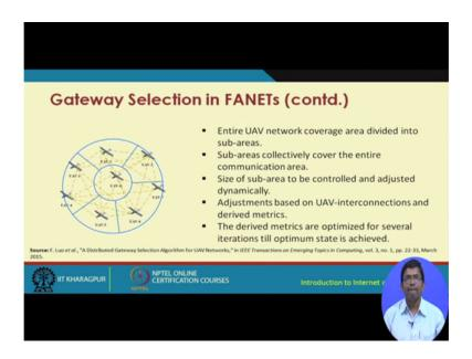
So, in this particular figure as we can see over here. We have a bunch of different UAVs, maybe working in a plane, functioning in a plane. And then we have one of these nodes which is designated as the gateway which acts as a coordinator, with all the other nodes in the same plane. So, inter UAV network coverage area will be divided into sub areas as
