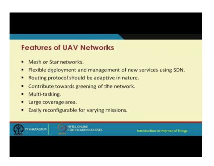
So, first thing is the topology. So, we are talking about a network which is highly dynamic, the topology is fast changing very fast changing, compared to this you know the terrestrial networks, compared to the terrestrial or ground networks. Because these are flying objects and they fly at very high speeds, the topology itself will be changing very fast. And the network itself will be moving together. And consequently the dynamic, dynamism in the topology is going to be very much.
