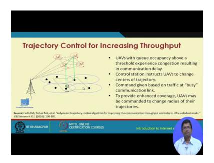
So, typically what happens is UAVs with queue occupancy above a threshold experience condition resulting in communication delay. The control station instructs the UAVs to change the centers of trajectory, and the command is given based on the traffic at the busy communication link.
