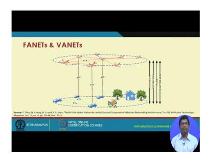
So, this is the flying ad hoc networks with a to a link etcetera, and then we have this v to v link over here in the vehicular network. And then here this connectivity shows the a to v link where, it is basically air to vehicle link.
