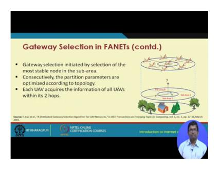
So, how do you select the gateway the gateway selection is initiated by the selection of the most stable node in a particular sub area? So, in a particular sub area the most stable node is considered. That must consecutively the partition parameters are optimized according to the topology where, each UAV acquires the information of all UAVs within it is 2 hops. So, flying ad hoc networks and vehicular ad hoc networks as you can see over here, there is a link up.
