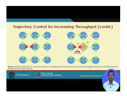
So, as we can see over here, in this figure we see that this is a grid like deployment of the UAVs. And the buffer occupancy or the queue occupancy are also shown in this green and red colored nodes. Great not nodes, but these grid colors green colored and red colored symbols.
