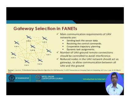
The main communication requirement of UAV networks are sending back of the sensor data, deceiving the control commands, cooperative trajection trajectory planning and dynamic a task assignments.
