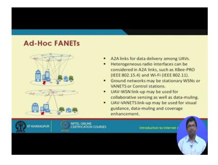
So, we have different types of links, we have the air to air links for data delivery among the UAVs. Then we have heterogeneous radio interfaces in the a to a links, using zigbee pro following 802.15.4 standard or using Wi-Fi 802.11 standard. The ground networks may be stationary sensor networks or vanets or contour stations, and the UAV-WSN link up may be used for collaborative sensing as well as data muling.
