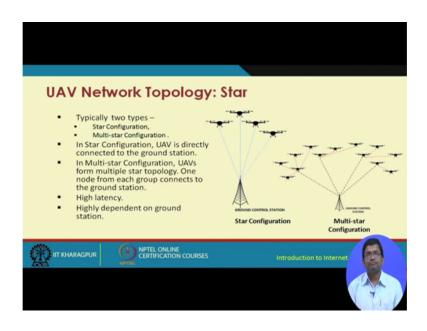
So, if you recall that initially we were discussing about the different topologies of UAV networks. So, we will start with the star topology. So, there are 2 types of topologies in star one is the basic star, and where we have this ground station. And these different UAVs basically connected directly to this ground station to form a star topology.
