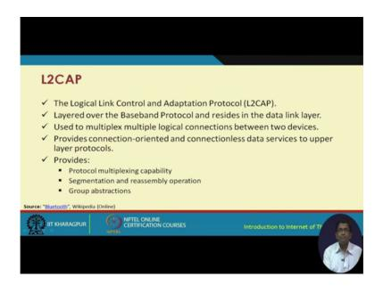
Then we have the L2 cap. And in the L2 cap which basically is on top of the baseband layer, functionalities such as multiplexing, multiple logical connections between 2 Bluetooth devices is functioned is made possible, in this using this particular layer.
