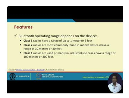
It supports one mbps data rate which is quite attractive short range high data rate communication is supported. In Bluetooth there are 3 types of radios that we will typically find and they all operate in different ways. We have the class one radios class 2 radios and class 3 radios. Class 3 radios have a range of up to 1 meter or 3 meters. Class
