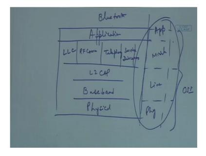
We have the L2 cap and then there are some different other layers and corresponding protocols that are supported in the top layers and then we have the application layer. So, these are the different layers in the Bluetooth protocols. I was telling you about cable replacement there are protocols such as RF comm protocols which will support traditional telephony, protocols that will support service discovery, protocols that will support other link layer functionalities such as LLC.
