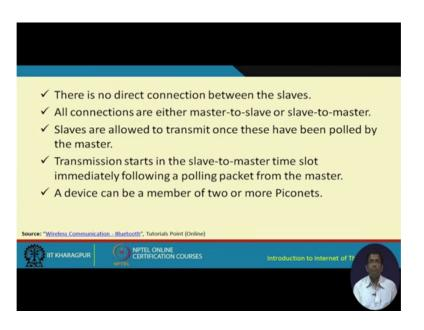
There is no direct connection between the slaves all connections are either through the master to slave or slave to master mode slaves are allowed to transmit. Once these have been polled by the master transmission starts in the slave to master timeslot immediately following a polling packet from the master and the device can be member of 2 or more piconets, and this is something that I explained earlier as well.
