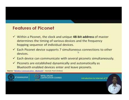
So, the master of the slave they use the 42 bit addressing. So, this is the addressing scheme that is used each piconet device will support 7 simultaneous connections to other devices each device can communicate with several piconets simultaneously. And piconets can establish dynamically and automatically as Bluetooth enabled devices enter and leave piconets.
