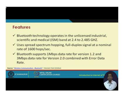
Bluetooth technology also like the previous ones like hart etcetera that we covered in the previous lectures operate in the ism band 2.4 gigahertz to 2.484 gigahertz, it uses spread spectrum hopping full duplex signal at a nominal rate of 1600 hops per second.
