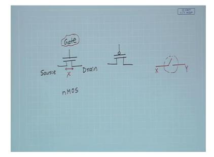
This is called the gate and the other 2 terminals one of them is source, other is drain, this is an example of an n MOS transistor the symbol and p MOS transistor is same where there is a bubble here, same kind.
