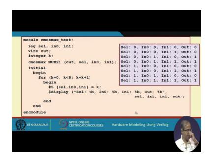
So, this again see here there are 3 inputs total right. So, we have written test bench similarly, but we have applied 8 pattern 0 up to 7 and this case assigned to select n 0, n 1 like this. So, we have printed the values of cell in one there should be n 0 actually n 0 n 1 and out. So, you see f select is 0 then n 0 is getting selected if select is 1 then n 1 is selected, 0 1 0 is getting selected right. So, it work as a multiplexer.
