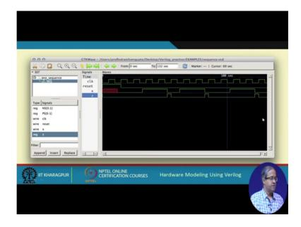
So, and then out delay we finish. So, the simulation output comes like this. So, this is I am not showing the whole of it a part of it, the clock is coming the reset you see the reset was activated initially to 1, and it remained till 15 it becomes 0. So, reset was one this is time 15 at time 15 it becomes 0 and after that it remains 0. So, my circuit starts operating from that point onward.
