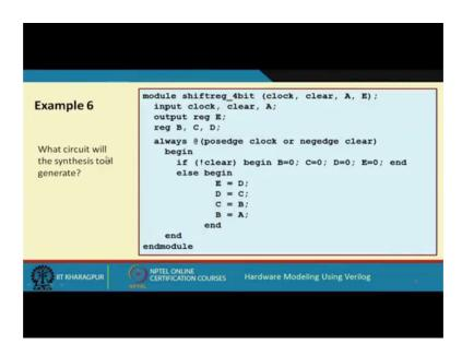
And it will bigger; well here our objective was to design a 4 bit shift register, suppose this was what we started to design.
