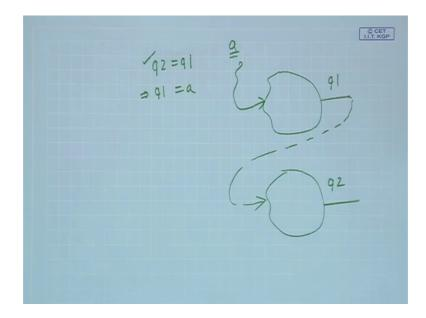
You see you can imagine, there were 2 flip flops, q 1 will be the output of 1 of the flip flops, q tool with the output of the other flip flop, first one you are saying that q 1 will be going to q 2 which means this q 1 has to be connected to the input of this q 1 will have to go to q 2.
