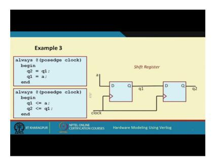
I just write it like this and below I write an description same description using nonblocking. Non-blocking assignment here let us try to understand; what will happen; here we have written q 2 equal to q 1 and q 1 equal to a; what does this mean?
