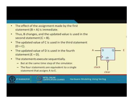
You have provided some specification, but the tool does some analysis and finds that well what you mean E is actually D equal to A, right. So, instead of a shift register, what it will be generating is nothing, but a single flip flop whose E equal to you know, D equal to E equal to final E. So, the A will be going directly to E.
