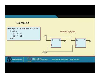
This is procedural block with a clock always posedge clock, here I am using a blocking assignment. So, what does this block mean this block means that whenever there is a positive edge of the clock you activate or start executing this what is this saying that you first assign a to q 1, then assign q 1 to q 2, right.
