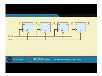
So, this is like the shift register thing. So, this is the shift register which will be trying to model like this, right and this is the description equal to D means.
