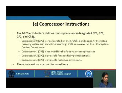
Next set of instruction is coprocessor instructions. The MIPS architecture defines four coprocessors, designated as coprocessor 0, 1, 2, and 3. CP0 is incorporated within the CPU chip and this also supports the virtual memory system and exceptional handling. CP0 is also referred to as system control coprocessor.
