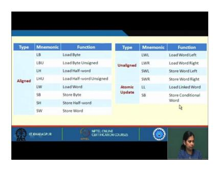
Now, we can see some more instructions; LB is load byte, this is load byte unsigned load half word and so on. And here for an unaligned one, we have load word left, load word right and similar way store word left and store word like right. And also for atomic update, we have load linked word and store conditional word.
