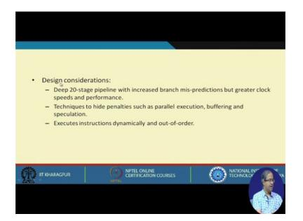
And here there was not much consideration on reducing the number stages in a pipeline to convert it into a RISC kind of architecture. It had a very complex pipeline comprising of 20 stages where the complex instructions were directly mapped and executed.
