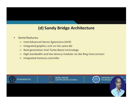
Then came the Sandy Bridge architecture. Here some vector extensions were made to the processor, and there was a separate engine that was called AVX advanced vector extension.
