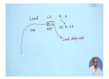
What I am saying whenever there is a load followed by its immediate use, as if there is a gap or slot coming here between the two instructions; this gap is called the load delay slot. If we do not do anything then the control circuit has to insert one stall cycle here.
