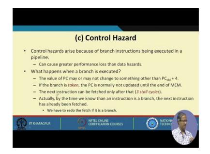
Now coming to control hazard; control hazards arise because there are branch instructions in a pipeline. Branch instruction means the next instruction to be executed can either be the sequentially next instruction or instruction from somewhere else. If the branch is actually taken it is a jump or a branch that is taken.
