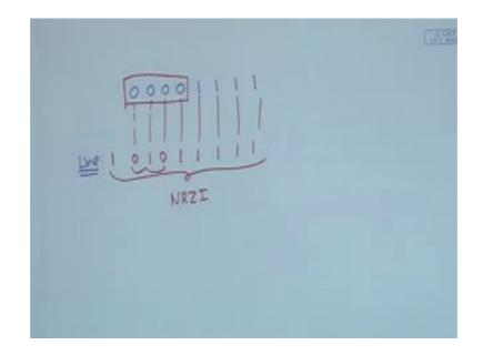
Suppose my data that I am transmitting is  $0\ 0\ 0\ 1\ 1\ 1\ 1$  and let say my line was initially at 1. The previous state was 1 and now this line is 0. You look at this table. Previous line state is 1, bit to be sent is 0, and the new line state will be 0. This way all the other bits are encoded.
