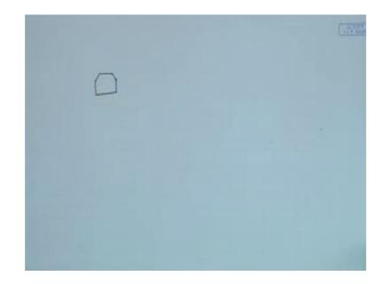
Beveled means it has a shape like this, right square, but the top two corners have a little curve. Now, this Type B plug traditionally was used to insert into an upstream port or a device, let us say printer.
