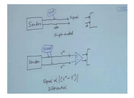
There are two ways in which you can send data. You can have two wires. One wire can carry your signal and the other wire can be ground. When you send the signal to the receiver, receiver should also know that this is your signal and this is your ground. So, you have to connect the signal in the proper order. This is sometimes called single ended connection.
