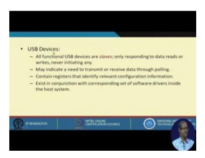
Conventionally all of the USB devices work as slaves. They cannot initiate any operations, they can only respond to operations that are initiated by the host. There are some registers inside the USB devices that can identify what kind of device it is and what kind of drivers it require, and so on.
