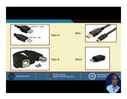
This picture shows you the Type A connector that you see mostly. It is a little elongated and flat. This is your normal connector and this is your receptacle. The normal connector will go inside the receptacle; and Type B looks like this. This will be your Type B connector and it will go inside a receptacle that looks like this.
