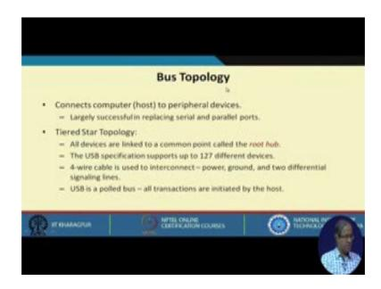
By bus topology what I mean is that how the external devices are connected. Inside the computer system, it is fixed. Now, how you can expand the capability so that you can connect several devices outside. You must have seen there are products called USB extenders available. You plug a device to the USB port and on the other side, you will be getting four USB ports.
