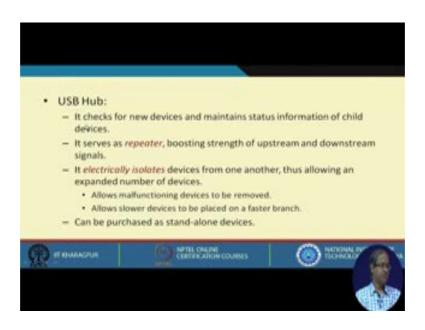
Talking about the USB hub, it checks the new devices that you are connecting to it and maintains status information. Like when you connect a new device to an USB port, that port will check what kind of device it is, and depending on that it will try to locate the driver that needs to be activated. If the driver is not available, the host will try to install that new driver.
