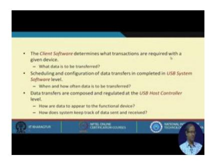
The client software determines what transactions are required with the device, what data is to be transferred. Scheduling and configuration of data transfer is completed in USB system software level. All data transfer gets completed here logically. When and how often data is to be transferred that is decided there, and either lowest level USB host controller data transfers are composed and regulated.
