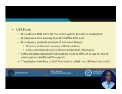
Now, you have host, you have hub, you have the devices. Talking about the host it is a device that controls the entire system, and this host is usually a computer or a laptop. Some mobile phones can also act as the host. It will be processing data arriving to and from the USB port. And it contains a sophisticated set of software drivers. Depending on the kind of USB devices that are connected, the appropriate drivers are selected and they are executed, so that data transfer can take place.
