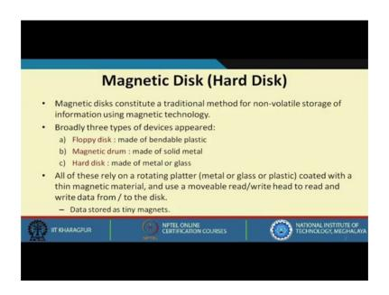
We start with our discussion on magnetic disks which has been around for several decades already. Now actually how does a magnetic disk work? Magnetic disks, as the name implies, rely on some kind of magnetic technology. There is some kind of ferromagnetic material coated on the surface of the disk, and with the help of some externally applied magnetic field we can change the orientation of tiny magnets on the surface.
