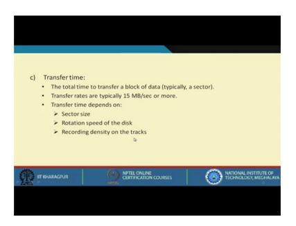
The data transfer rate in bytes per second or kilobytes per second whatever you say, is the total time required to transfer a block of data, say a sector or a track, in a disk. The typical transfer rates are typically of the order of 15 megabytes. The transfer time depends on several things, the sector size, rotation speed of the disk because faster the disk is rotating my speed will be higher, and also recording density on the tracks.
