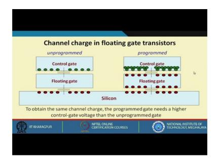
By applying some voltage on the control gate you can inject some electrons or some charges within the floating gate like this. Suppose when there is no charge on the floating gate, when you apply some normal voltage on the control gate some electrons will be attracted on the channel just like a normal transistor and between the source and drain a current will be flowing.
