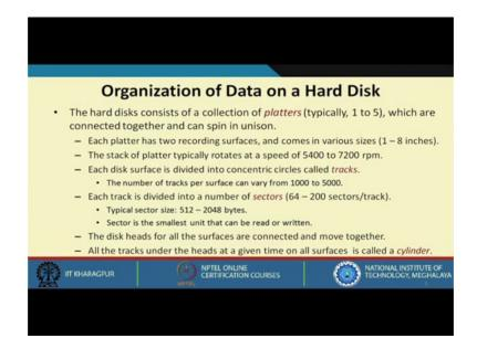
Let see how data are organized on a hard disk. As I had said each disk is called a platter, platter is a circular hard material which is magnetically coated typically on both the sides. Now a magnetic disk unit as I had said can contain more than one platter which rotates all simultaneously.
