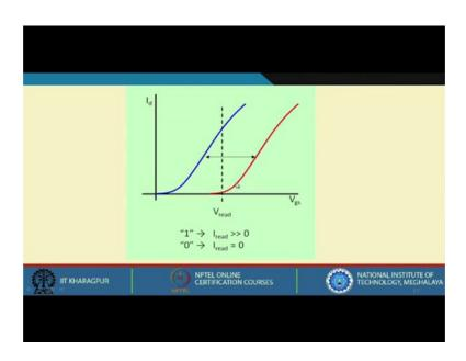
These are the characteristic curves. As you can see for one state the current will be very less, and for the other state the current will be quite high. So, just by measuring the current you can sense that in which state your device is in, 1 or 0.
