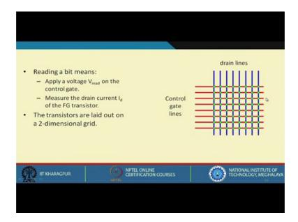
Now, when you talk about reading a bit it means you apply a voltage on the control gate and measure the drain current whether the current is flowing or not; and typically this transistors are laid out on a two dimensional grid. These red and blue lines are on two different levels they are not touching, and the transistors are fabricated at the junctions; one is the drain other is the source, this is the gate and transistors connected like this.
