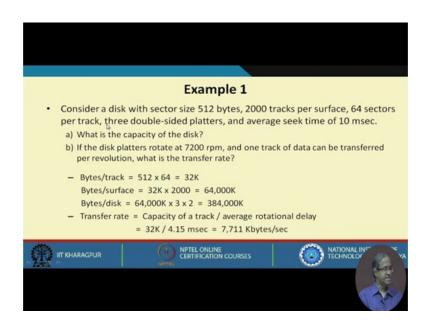
Let us work out a simple example. Let us consider a disk, where the sector size is 512 bytes, there are 2000 tracks per surface 64 sectors per track, and there are 3 platters double-sided, so there are 6 surfaces, and average seek time is 10 millisecond. The first question is; what is the capacity of the disk and the second question is if the disk rotates at 7200 rpm and we assume that one track of data can be transferred per revolution what is the transfer rate?
