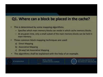
You remember we said that we will be answering 4 questions. The first one is, where can a block be placed in the cache? Firstly, where my block will be placed in the cache is determined by mapping algorithms. This specifies which main memory block can reside in which cache memory block. Which block of the main memory will be in which block of the cache must be determined using some mapping technique.
