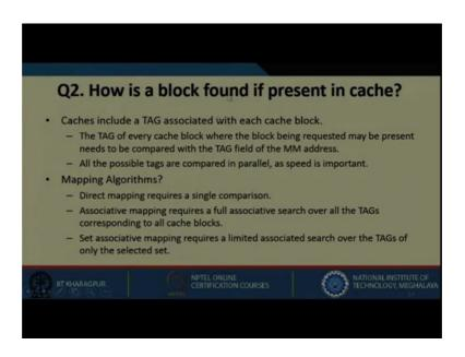
So cache include a TAG associated with each cache block. The TAG of every cache block needs to be compared with the TAG field of the main memory address. So, the TAG field of the main memory address is compared with the TAG of every cache block; all the possible tags are compared in parallel as speed is very important.
