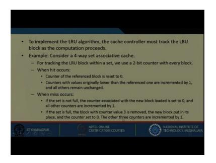
To implement LRU algorithm the cache controller must track the LRU block as the computation proceeds. We need to keep track of the LRU block. A 2-bit counter can be used with every block for this purpose, as explained.
