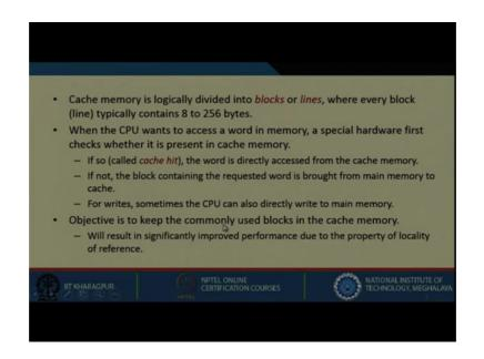
Cache memory is logically divided into blocks or lines, where every block or line typically contains 8 to 256 bytes. When the CPU wants to access a word in memory, a special hardware first checks whether it is present in cache memory. If so we call it a cache hit and the word is directly accessed from the cache memory. If not, the block containing the requested word is brought from main memory to cache memory.
