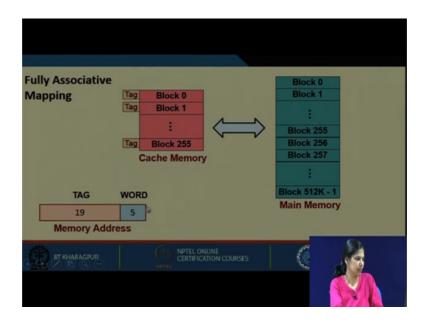
So in fully associative mapping we have total of 256 blocks in cache memory. Any 256 blocks from main memory can be brought in here, and which block of main memory is here is determined by this 19 bit TAG field.
