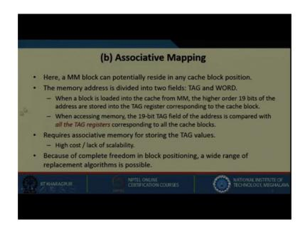
Next, let us move on with associative mapping. Here a main memory block can potentially reside in any cache block position. In case of direct mapping, we have seen the problem, even if there is space we cannot keep a block. We cannot bring any block from main memory because of that condition. So, here in this associative mapping this condition is relaxed.
