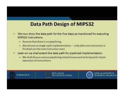
First, the data path design of MIPS. Individually, we have seen that how we are actually executing a particular instruction, what are the micro-operations that are required to be executed. How the data path is actually designed we will see here.
