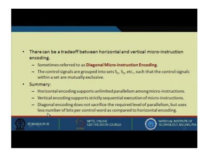
Let us say we have a total of 100 control signals. In case of horizontal control unit design we require 100 bits for each control word, but in this case we require only 7 bits. So, at a time only one control signals can get activated because we are encoding using just 7 bits, earlier for horizontal it was 100 bits, but for this we only require 7 bits. So k bit control word can support up to  $2^k$  micro operation. So, if you have 100, then only 7 bits will suffice.
