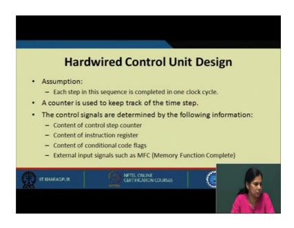
In hardwired control unit design there is an assumption that each step in the sequence is completed in one clock cycle, but remember one thing that when we are reading something from the memory it may not be completed in one clock cycle. We cannot ensure that if we are reading from memory it will be completed in 1 clock cycle, but this is an assumption that we have made. A counter is used to keep track of the time step.
