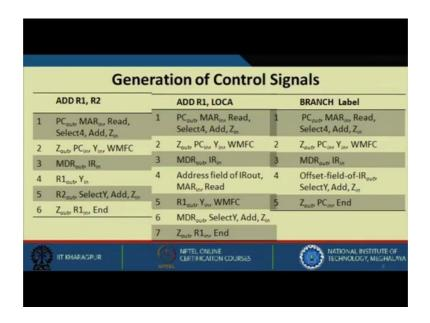
So, keeping the flexibility of this hardwire simple instructions are basically implemented using hardwired control unit design. Let us now see these 3 instructions together. These are the control signals required for ADD R1, R2; ADD R1,LOCA; and BRANCH Label. So, at various time steps following control signals are getting generated.
