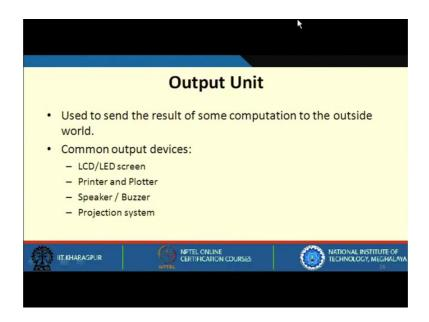
And the output unit is used to send the result of some computation to outside world like printer is used to print the data, LCD screen or LED screen is used to see the output on the screen, you have speakers, you have projection system that are also used as an output unit.
