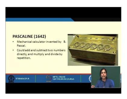
So, this is the first mechanical calculator that was invented by B Pascal. So, this particular calculator could add only two numbers, it can only add two numbers or it can only subtract two numbers. And if you wanted to do multiplication and division, it could have been done by repeated addition or repeated subtraction.
