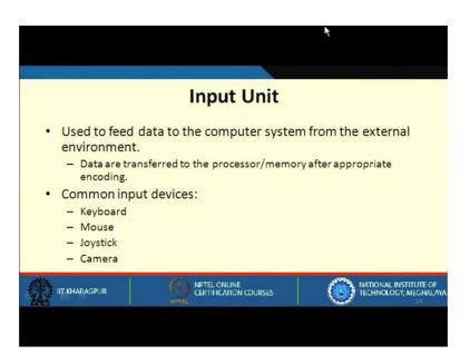
Coming to the input unit, it is used to feed data to the computer system. The commonly used devices are keyboards, mouse, joystick and camera.
