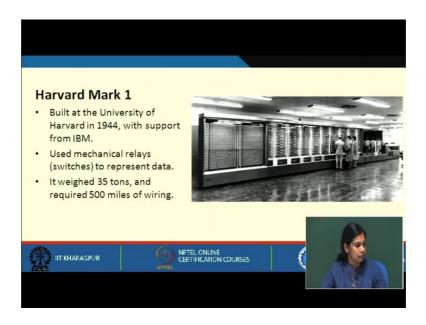
Next was Harvard mark 1. This was built at the University of Harvard in 1944, with support from IBM and it uses mechanical relays and off course, some electric signals were also used to work with the relays to represent the data. And it also weighted 35 tons, and required 500 miles of wiring. So, these are the computers which were built in the early stages.
