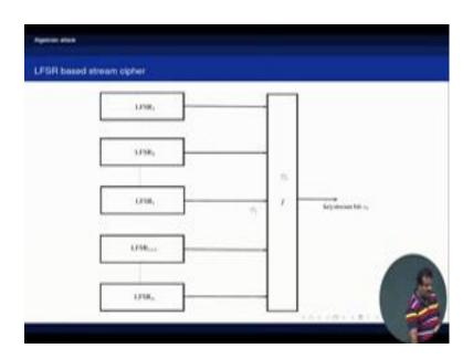
So, this is we have seen if it is LFSR based stream cipher, we have n LFSR which is taking the input to the non-linear function f, and we are generating the key stream.
