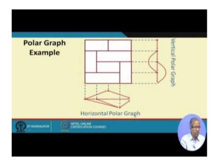
Let us take this example. So, this is a layout or a floor plan, this is the horizontal polar graph. In the horizontal direction you see these are the vertex, what does the vertices indicates? The vertices will indicate in each place where you have a vertical line, here I have a vertical line here, next I have a vertical line here in this block here I have a vertical line here in this block, here I have a vertical line here, and at the end I have a vertical line here.
