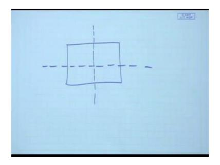
Slicing structure means it is like a rectangular dissection like let say suppose I have a floor plan, say there are many blocks. Dissection means I can cut the floor plan either by a vertical line or by a horizontal line like this, I can cut it into 2 parts this are called dissections. So once I do a dissection I divide the floor plan into 2 smaller floor plans right.
