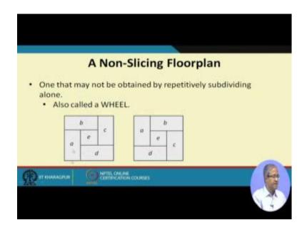
Now, these are the example of a floor plan you can see; here also we have some blocks which are very nicely placed, but you cannot slice them. As you can see you cannot have a continuous vertical or a horizontal slice that can partition. This floor plan this is something which is called a non sliceable floor plan and a topology like these 5 blocks which are oriented in this fashion this is called a wheel.
