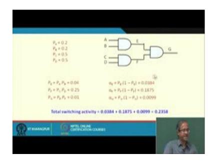
But now suppose we map the gate in this way, where the gates are in 2 level obviously, delay is less the gate will be faster, but with respect to power let us see, the same probability values. Now P values will be like this, P will be similarly P A P B 0 4, P F will be P C into P D 0.25, P G will be P into P F 0.01.
