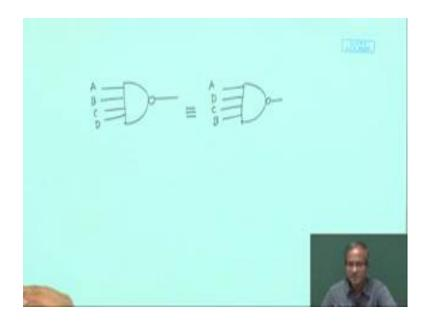
Normally when we have a multi input gate so, we connect ABCD like this, suppose we have another scenario same gate, but we connect the gates like say ADCB. Now because the nand function is commutative, where you can easily say that these two are equivalent, these two are equivalent functionally of course; but you may also be tempted
