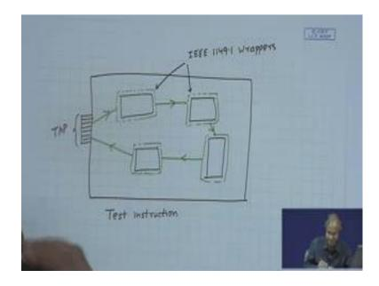
Let us say there are several chips, and on the edge of the board I have some kind of a connector through which I can feed some signals.
