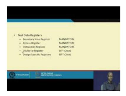
Now, among the special registers, these 3 registers are mandatory. You must have the boundary scan registers alongside the input and output pins. You need to have a BYPASS register in case you want to skip a chip; you need to have a instruction register to store the test instruction.
