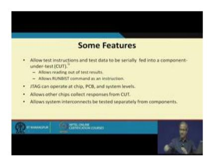
So, some of the features of this boundary scan technique is as follows. Here we apply tests as some kind of instructions, like let me show you the overall prospective. Like I have a printed circuit board I have board. So, there are several chips which are residing on the board.
