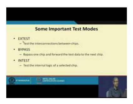
Now, here we shall be show you 3 of the important test modes of the boundary scan, there are other modes also. EXTEST BYPASS and INTEST, now the EXTEST mode is used to test the interconnections between the chips - BYPASS mode is used to skip one chip and go to the next one. And INTEST is used to test particular chip; that means, the internal logic. Let us look at the basic concepts one by one.
