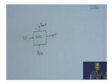
So, from the left side you have a signal let us call it in, and the right side there is a signal called out. So, on from bottom there can be a signal S in and from top 3 can be a signal S out.
