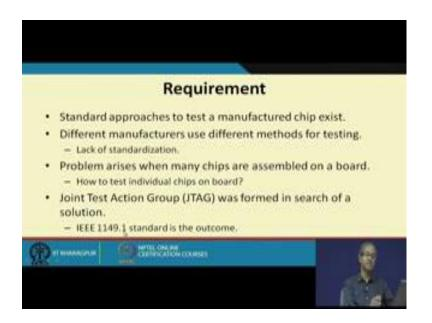
So, this is actually one of the standards like I was talking about. So, you know how manufacture chip can be tested. We looked at several methods test generation dft and so on. As I said different manufactures may use different methods for testing. So, there is no standardization or there was no standardization. So, when several chips are assembled on a board. So, how do I test the individual chips, why they are designing on the board.
