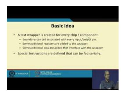
So, I said the basic idea is to have test rapper, for every chip or component that is manufactured now. In fact, the EDA tools using which you design the chips, they have a instructions a single instruction and instruction to create the rapper.
