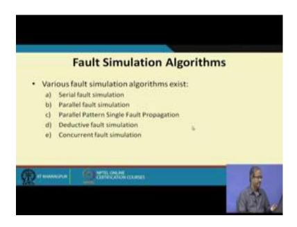
Now, the various fault simulations algorithms can be classified as follow, let the first 1 is the 1 that the naive approach we just now saw, the rest 1 are some kind of faster versions. So, we shall see how they work.
