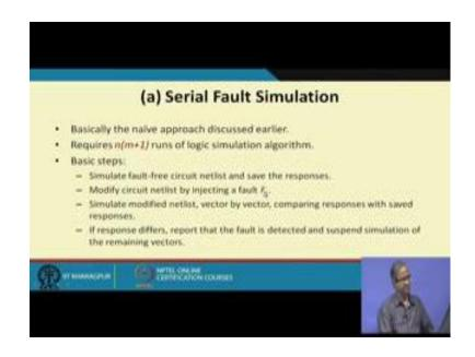
So, serial fault simulation we have already seen this is the naive approach. So, we have seen that it requires so many runs of the logic simulation algorithm, where n is the number of test vectors, and m is the number of faults. So, they will be m number of faulty circuits and 1 faulty and 1 fault free circuit, so many simulations we have to carry out for every test vector.
