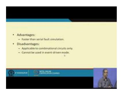
So, this method is clearly faster than serial for simulation, but the disadvantage is that it is applicable to combination circuits only; and it cannot be used event driven mode, because you are injecting different faults in different bits you cannot identify the events like that that I have to simulate this part not that part, but to simulate for all the faults.
