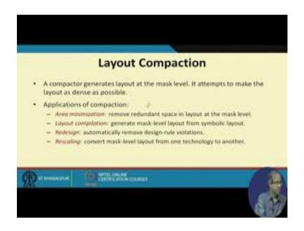
Now layout compactor what it does? It generates or it reduces the area of a layout at the mask level well. Compactor is general it can generate the layout from this stick diagram also like what I have said or given a layout it tries to reduce the area by bringing some rectangle closer to each other. See the idea is this you already have the design rules,
