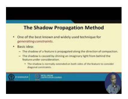
Constraint graph means given a number of blocks, blocks means rectangles I am talking about here in this context. So, what are the constraints separation their connectivity and so on. So, one of the very interesting methods of generating this kind of constraint graph is something called shadow propagation. Shadow propagation means the idea just follows suppose I have the layout with me. So, I am using an imaginary source of light.
