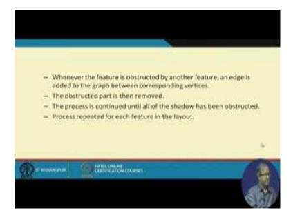
So, the constraint on all the sides similarly up similarly down, they will be considered in all directions. So, whenever the feature is obstructed by another feature we add an edge this is the idea, and the obstructed part is removed.
