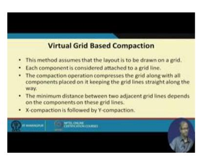
Then we come to something called virtual grid based compaction. So, here we are imagining a grid on the layout surface. So, where assuming that the components are all attached to a grid, it means it is something like this.
