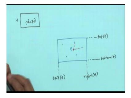
Suppose I have a cell. This block I am placing I call it v. This center point center of this cell, I call it the coordinate xv and yv right. Ve denotes the set of cells which are connected to net E. And left right bottom and top denote the coordinates of the 4 boundaries of es bounding box. So what does this mean? Let us explain.
