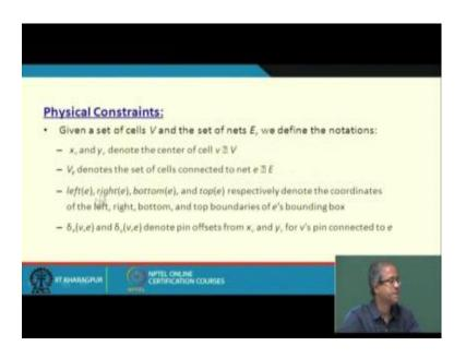
So, the physical constraint let see what these are. Given a set of cells V in a set of nets E we define xv, yv to be the center of a cell v, there should be, belongs to see this symbol has not come small v belongs to capital V. So what does this mean?
