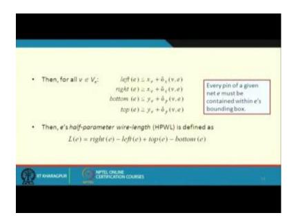
Let us look at the constraints now. So the physical constraints say the first set of constraints they tell you that every pin of the net e must be within the bounding box. These are captured by these 4 constraints. Left e must be less than equal to the x coordinate of the center plus that offset, for that pin e. For some pin for every v belonging to this net the v must be this. Similarly, right one should be greater than equal to the y
