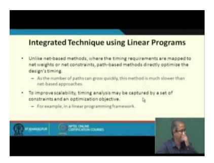
So, these are some of the methods which have been used, but the integrate approach is interesting here, the entire process of optimization you are expressing mathematically and you are using some kind of a solver like linear programming solver LP solver to get a solution to the problem. That, what will be the placement such that these constraints are met. So let see on that here how this works.
