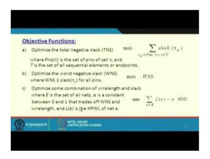
So, the objective function can be 3 types, 3 of them are shown here. You can add some more. First one is to optimize the total negative slack. Total negative slack can be expressed like this Pins tau is a set of pins of a cell tau, and T is the set of all sequential elements or endpoints. So you calculate the slack of all system. One thing is not mentioned if it is total negative slack, we will also have to mention another condition that slack tau p should be less than equal to 0, right.
