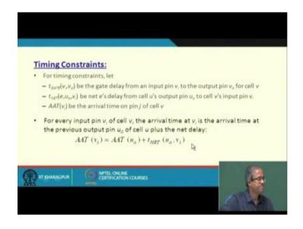
So, timing constraints you can similarly add like this. So some notations T gate v I, v o is this defined as the gate delay from a input pin v i to the output pin v o of a particular cell. And T net e, u o, v 1 is net is delay, delay of a net from cell u's pin some output pin u 0 it is coming from a cell u, u 0 is the output pin and it is going to the input pin of v, it is called v i. That net delay and AAT you get from static time analysis. This is the actual arrival time on pin j.
