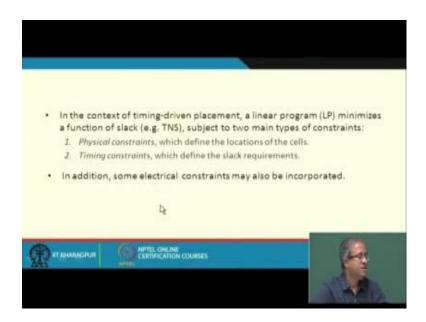
So, how does it work? They actually specify 2 kinds of constraints. One is called the physical constraints those are the placement so where the cells are located and timing constraints that concerns the slack values. So in addition you can also incorporate some additional constraints some electrical constraints if you want, but we only talk about these 2 here physical and timing.
