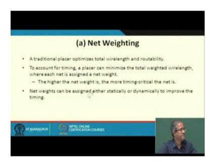
Let us look at some of the existing methods which have been proposed for this net weighting how they make the estimates. So a traditional placement tool that we have seen earlier this optimizes just the total wire length and routability, whether there is sufficient space for routing.
