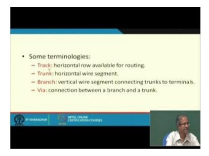
So, there are some terminologies that we use in channel routing. Track, track is a horizontal row that is available for routing. Trunk is a horizontal wire segment, so one net maybe connected using multiple trunks. Branch is a vertical wire segment that
