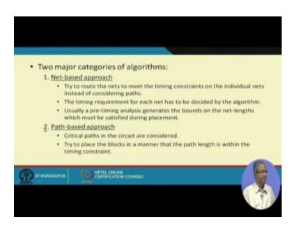
So, the algorithms broadly can be classified into 2 classes: 1 works on a net by net basis. So, recall what is the net? A net is a connection of pins, which have to be connected; they belong to the same means equi potential net in that sense. So, in the net based approach here we try to route the nets to meet the timing constraints individually on a net by net basis, we do not consider the paths.
