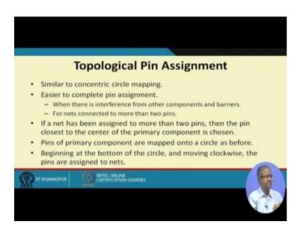
So, topological pin assignment is an alternate method which is quite similar to concentric circle mapping in. In fact, it is a little easier so here you can just handle nets which is assigned to more than 2 pins.
