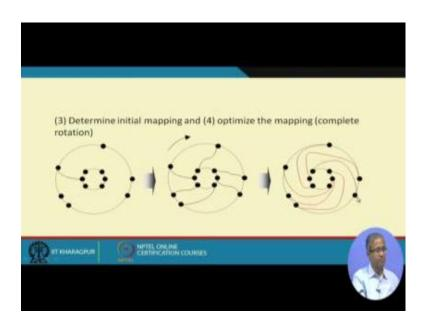
How? Then we try to find out initial mapping. First let us say initial mapping says, this pin is connected to this pin, this pin must be connected to this pin, this is connected to this pin. So the ordering is there. So now, you try to rotate them in some way. You see this is a bad rotation, if you rotate this pin to here then I have to connecting using long wires. So you try to rotate the pins in a way rotating in a way, such that the interconnections become simpler.
