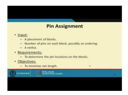
So, this is actually what I mean to say in this last point. So in this a pin assignment, the input is a placement of blocks, number of pins on each block. Possibly in ordering this ordering may or may not there. This ordering means well you know that there are 3 inputs and 2 outputs.
