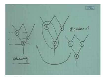
For example suppose I have got in a data flow graph, I have got some graph like this. Suppose these an operation. How many adders do I need, how many adders? Only one it suffice, because this one and this one these additions, are not being done at the same time; therefore, I can very well mark this function unit, but that would not have been possible, if my operation was something like this right.
