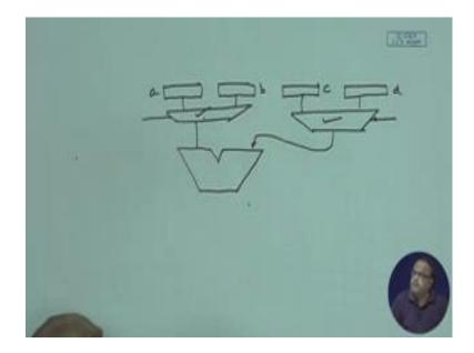
For example if I have, say some operator is here, some ALU is here, and the ALU is getting data from variable a, it can take the left input, can take from variable a or b or c or d, say the right input comes from. So, c or d comes to multiplexer, here I put a mask. And from this multiplexer I take this data, and this one also comes to a multiplexer with some control, and I can take data from here. So, a or b comes here and c or d comes here.
