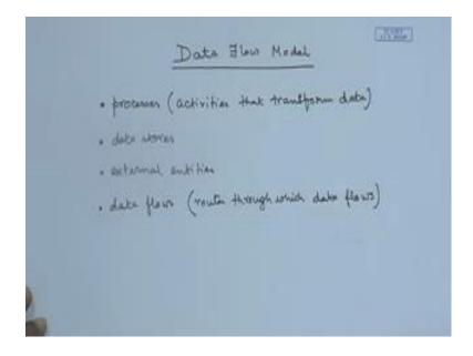
Now data flow is very common, and very natural. In data flow model, we are not looking at the states, we are looking at how the data is flowing alright, across the system, and we will show a particular type of example.
