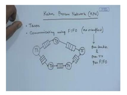
A particular data flow network known as the Kahn process network, or KPN. A lot of research is going on now, modeling systems using KPNs. Now here each component of the Kahn process network is modeled as a task. So, we have got some tasks. Now this task can be programs or processes alright, and the tasks are communicating among
