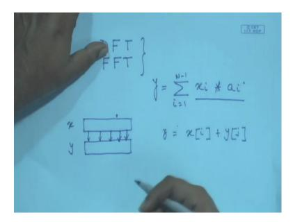
Now, this sort of this type of operation is present in different DSP applications like say Discrete Fourier Transform, Fast Fourier Transform, these are very standard signal processing applications, all of these have got operations of this form or a j, it could be 2, it could be 2 summations etcetera.
