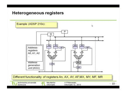
So obviously, that is another advantage of the DSP processors where we can utilize as we did in our earlier example that we worked on where we did this MX and MY were being fetched the two values of w value and a value were being fetched simultaneously. That is possible because we have got multiple memory bank or memories. So, that is another advantage another measure that adds to our efficiencies.
