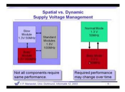
One thing that we can think of is spatial and dynamic supply voltage management. All the first parts of the circuit need not be given a uniform Vdd, the same Vdd. We can have say for example, this part is a very busy module and most this is a hotspot, most of the computations have been done here in the red one. So, I want to make it faster. So, I put it at 3.3 volt and 200 megahertz. Now if I go from this sort of curve I can say that at the particular Vdd what is the frequency that I can take.
