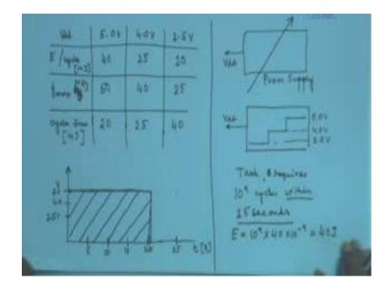
Suppose I had a Vdd box here, a power supply box for the Vdd; some Vdd comes out of this, it would be ideal if I could continuously control it, if you do linearly controllable for every point. But that is practically not very feasible to have such continuous supply. For that most of the systems that we have we have some discrete levels of say may be 3 levels of power supply, see 5 level, so whatever.
