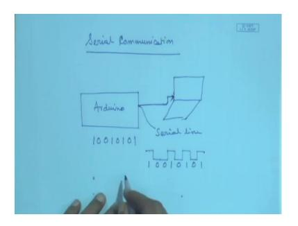
The serial communication whenever I have got the Arduino board here and I want to connect to my PC; I like to connect to this. Now this I can do through a serial port, serial line and how is that serial; suppose some data pattern 1 0 0 1 0 1 0 etcetera 1, 2, 3, 4, 1; I want to send, then in the serial mode it will send as a big pattern; in the parallel mode all of you know that it goes straight, but here it will be 1 then 0, 0, 1 then 0 again 1, 0, 1, so this will be 1, 0, 0, 1, 0, 1, 0, 1.
