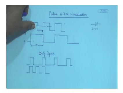
But we can play a trick for that; we have got a thing called pulse width modulation, some of you might be familiar with this. Suppose I want to say that LED that was there, I want to supply 2.5 volt; I cannot directly to the digital pin I cannot send 2.5 volt.
