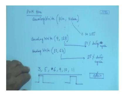
So, in Arduino we have got the command analog write; the pin and the value. The value is the duty cycle for the PWM pins; for the PWM pins we will write analog write and this value is between 0 to 255; that means if I write analog write pin number 9, 128; that means, pin number 9 will be fade with the pulse with 50 percent duty cycle.
