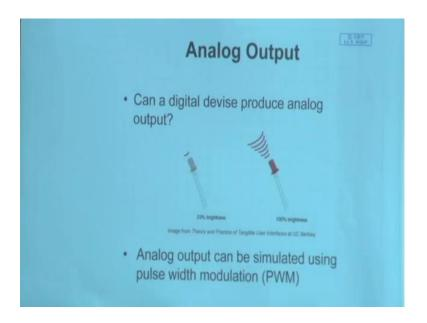
Now, next question that we would like to see is that suppose I have got an LED; I want to of course, with this LED is connected to pin 13. So, I can make it on or off through digital output; digital write, but if I want to make it glow in a continuous form that mean say with 23 percent brightness for some input, 100 percent brightness for some input; how can we do that? So, first of all we are talking about the analog output, how can we
