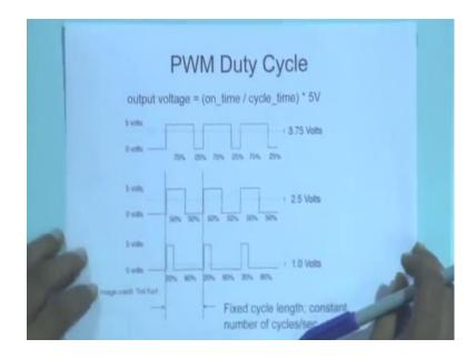
So, here once again let us look at this I think this is visible; the output voltage that will be getting ultimately is on time; this on time by the cycle time, the cycle time is 100; times 5 volt. So, here you can see 75 percent of the time is on and then it is off, so the output voltage of this will be 75 percent of 5 volt; 0.75 into 5. Here this is a 50 percent duty cycle, so it will be 2.5 volts; here it is 20 percent duty cycle, so it will be 1 volt.
