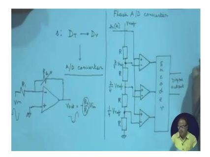
Now, discretization is nothing but again I will is a signal I am discretizing that from D T to D V. So, I am taking two from some continuous domain toward discrete domain and that is being done with a A to D converter alright. Now here there are different types of A to D converter. First we are trying to describe one type of A to D converter that is known as flash A to D converter.
