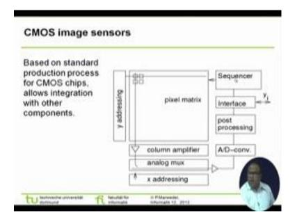
On the other hand there is another one which is a CMOs based image transfer image sensor, I am sorry, where we have got an area of image is being sensed in the rows and the columns and we are having an analog multiplexer and we are doing the analog to digital conversion and all those things.
