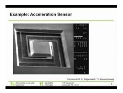
Here is an accelerometer, nowadays this accelerometer comes in different even in our phones where we have good gyroscopes and all those, but you never thought, what is the sensor that has gone inside? So, that will have to find out. So, actually there is a sorry there is a small thing that moves this thing and the rate at which it moves from there we find out what is the acceleration. So, there will be it can be a magnetic sensor.
