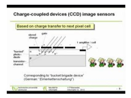
Now, there are different ways of image sensors which are there often in cameras, now they actually come in 2 forms, one is say CCD image sensors where we have got the charge coupled device here and depending on the light there is there is a physics that takes place in the semiconductor level and based on the charge transfer this works.
